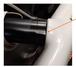
The issue may be caused by wear to the spacer that is located between the black jib tack bar and the hull.
