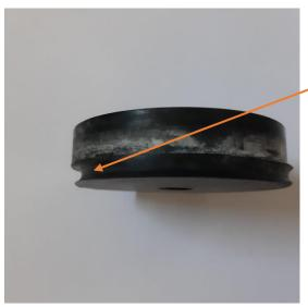
Over time, the downhaul rope cuts into the spacer and creates a groove that then traps the rope causing excess friction.
